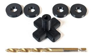
To load a 120 spool, you need to first slightly enlarge the hole at both ends of the 120 film spool (as well as a 120 takeup spool). This can be done very easily, in less than a second, with a drill. Just drill out the existing hole, no deeper than the original hole. If you wish to do this in the field, with no drill
