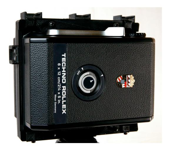
Its chief advantage over the Horseman 120 back is that it features a full 120mm wide aperture, for reduced horizontal masking when mounting MF3D slides. Other advantages include an extremely smooth advancing mechanism thanks to an oversized roller and exceptional machining of the advance gearing, and amazing German build quality.
