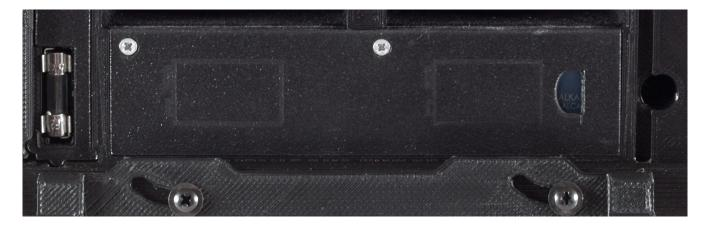
The Mercury takes two 9V batteries. We recommend using name brand Alkaline batteries. Lithium batteries last much longer, but have less power and can lead to inadequate triggering. Do not use rechargeable batteries—they don't have enough amperage, and their internal circuitry will likely shut them down due to the Stereo 12's unique circuitry.
