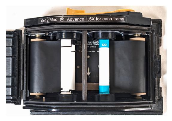
Now load the backing paper as usual: pull it around the front of the film insert, then back around the takeup spool. Use the back's advance lever to begin to wind the paper around the takeup spool.
